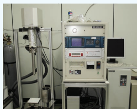
Gravimetric sorption system
