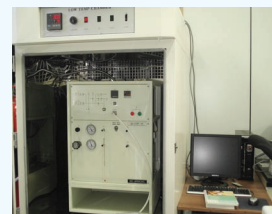
Volumetric sorption system
