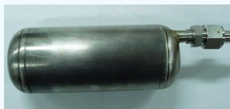
MH tank utilizing high-performance hydrogen storage alloy (1.4kg)
