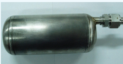
MH tank with 1.4 kg of HSA
