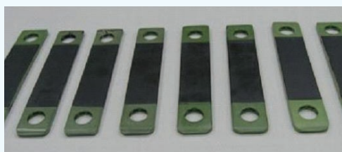
Close-end type of steam electrolysis cell
